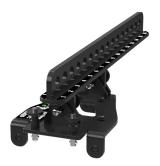
The T12GRID is used to vertically array TORUS for up to 6 cabinets. Cabinets may be flown from the T12GRID inverted allowing stereo arrays to be mirrored with the high frequency horn either to the left or the right.
