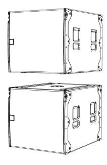
Remove the pins from the front SXCF115 to release the links.
