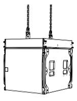
Replace the pins to link and lock the SXCF118 securely to the WPSGRIDt.
