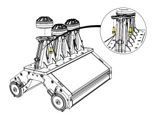
Remove the socket cap fasteners from the backplate to replace the diaphragm.
