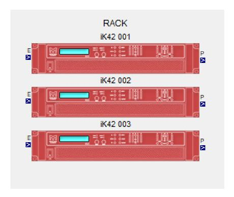
Presets are added to the amplifiers using the preset manager. Right click an amplifier to access the preset manager.
