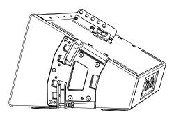
There are two mounting plates, one on either side of the cabinet. Decide which orientation you want the HF horn (left side or right side). Align the two pins and place the SBAR40 onto the mounting bracket.
