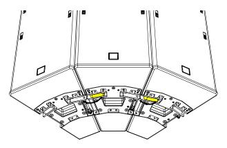
Replace the pins to link the bottom of the cabinets together.
