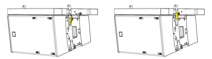
ft the array to a height where the next cabinet can be positioned underneath. Either lift the cabinet into position or lower the T12GRID onto the cabinet below.
