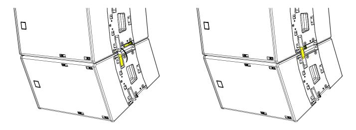
Repeat the process until the desired amount of TORUS have been vertically arrayed.
