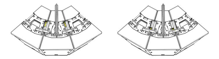
Lift the array and remove the rigging pins on the bottom of the array. Rotate the links into position.
