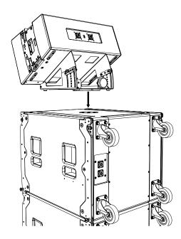
Remove the M20 handwheel from the stowing plate and secure to the M20 pole mount through the hole on the base plate of the GSRIG1530
