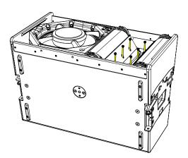
Remove the horn assembly from the cabinet and place driver side up on a flat service.
