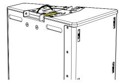
Two mounting options are available depending on the configuration. The HRIG100 can be mounted directly to a TORUS or between two cabinets.
