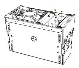
Remove the 6 posi drive screws from the horn flare.
