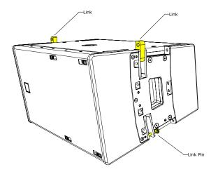
The fixed angled enclosure can be arrayed vertically and horizontally and deployed in various configurations with additional hardware.
