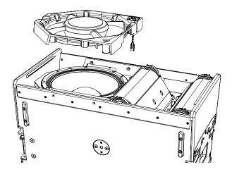
Remove the LF driver and disconnect the spade terminals.
