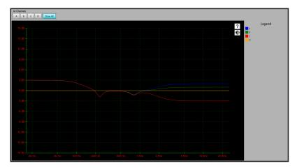
The high-pass filter is available on the Output EQ section for use with a subwoofer.
