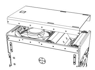
Remove the socket cap fasteners from the LF phase bung in a star pattern. There are 8 around the circumference of the driver and 2 on the side next to the HF horn. (6mm hex tool).
