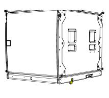
Lift the array to a height where the cabinet can be positioned underneath. Either lift the cabinet into position or lower the array onto the cabinet below and secure both side using the TORUS rigging pins.
