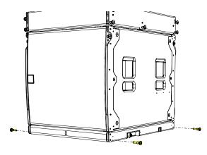
Rotate the four links on the T12TRIG and align them with the SXCF118 rigging hardware.
