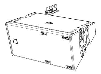
Turn the handwheel and tighten securely.
