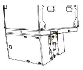
Replace the rigging pins to secure the cabinet to the T12TRIG.
