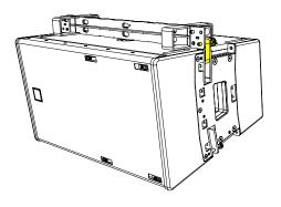
Lift the array to a height where the next cabinet can be positioned underneath. Either lift the cabinet into position or lower the T12PB onto the cabinet below.
