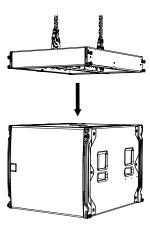
Remove the pins from the from SXCF118 to release the links. Rotate the SXCF118 links and line them up with the pin holes in the WPSGRIDt.
