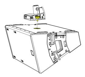
Turn the handwheel and tighten securely.
