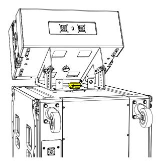
The angle of the GSRIG1530 can be adjusted before adding more T8 cabinets, by removing the rigging pins from the side plates.  $\,$
