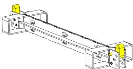
Secure the T12PB to the bottom of the array using the rigging pins from the bottom cabinet
