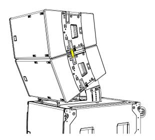
A maximum of 3 can be arrayed on top of the T8GSRIG. And any Martin Audio subwoofer that has an M20 pole mount can be used with this accessory. SXC(F)115, SXC(F)118, SX218
