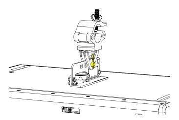
Secure the cabinet to the truss.
