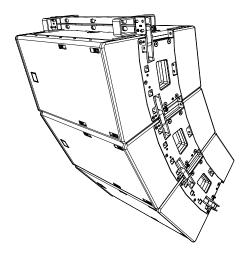
A second T12PB can be linked to the bottom of the array and used to achieve angles that are not possible with a single T12PB. The configuration can also be used to secure the array to stop it moving.
