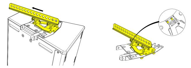
The HRIG100 is only secure when the two locking pins have been inserted and locked into place.
