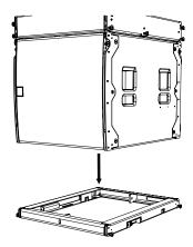
Remove the rigging pins from all four corners of the T12TRIG
