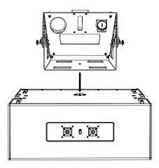
Remove the M10 handwheel from the stowing plate and secure to the plate through the mounting hole on the top plate of the GSRIG1530
