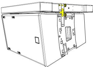
Remove the rigging pins from the cabinet below, rotate the links on the cabinet above and insert the rigging pins to secur
